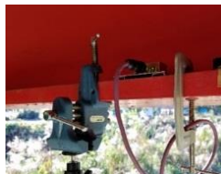
(a) MEMS sensor and the universal joint clamp connected with a carbon rod.
