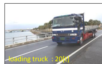
b) Loading test and prepared truck
