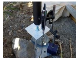
(b) Contact displacement sensor using a carbon rod connected with a universal joint clamp
